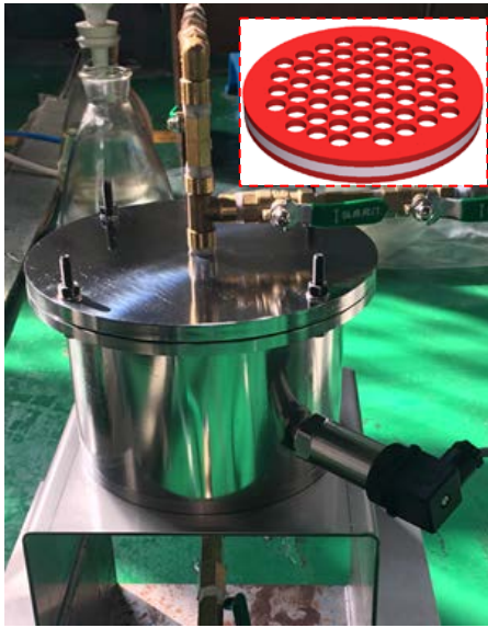
FIGURE 1 Example of one-dimensional transverse permeability test mold: (a) Tool with pressure sensors near the inlet and outlet. (b) Perforated plate.
