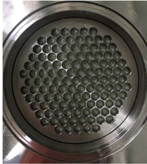
FIGURE 1 Example of one-dimensional transverse permeability test mold: (a) Tool with pressure sensors near the inlet and outlet. (b) Perforated plate.
